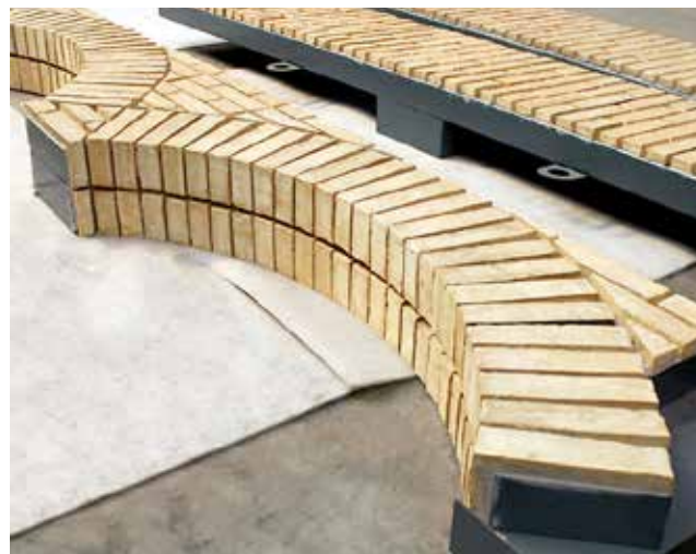
Structural arch with bonded slips
