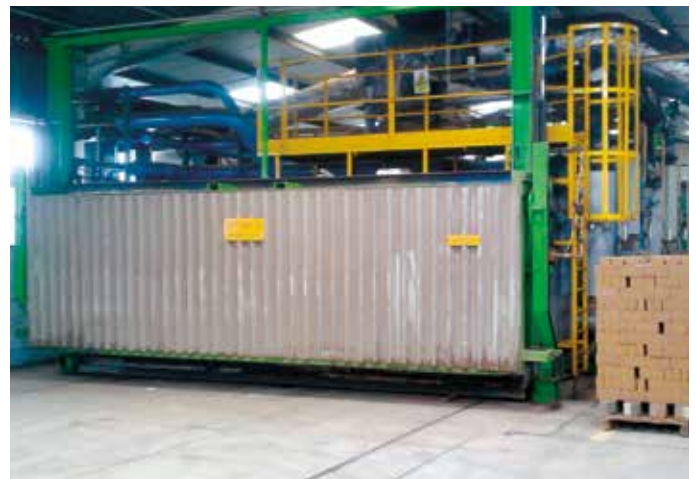
'Intermittent / Shuttle' kiln
