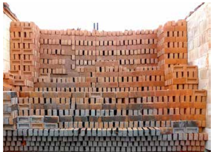
Bricks in a Traditional Open Square Kiln
